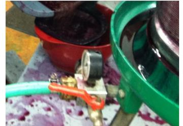
\* There is an automatic blow-off on the intake valve that will spray water if pressure gets too high; do not rely on this to manage pressure, turn down water at source if blow-off starts spraying or you risk damaging or destroying the bladder (and your wine)!
